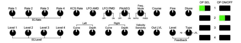
The right part of the control panel is the operator section. It behaves differently to the common section in that parameter changes only apply to the selected operators.
