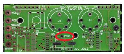
Use a minimum of 470 ohm resistor in series to a jack socket. (470 ohm to 1800ohm will work fine) You can now use this output as a arp clock for the juno or other devices.
