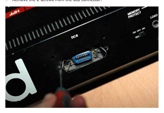
**Step 4.**□ Pull-out the dcb connector and remove the wires from the connector:
