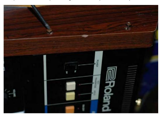
**Step 3.**☐ Remove the 2 screws from the dcb connector.
